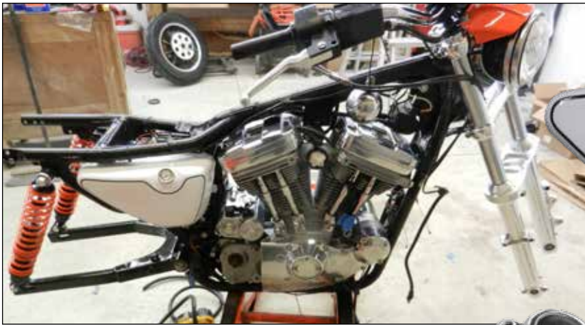
Forks were polished and the oil tank was painted white to replicate a flat track side number panel to match the white battery cover on the other side
