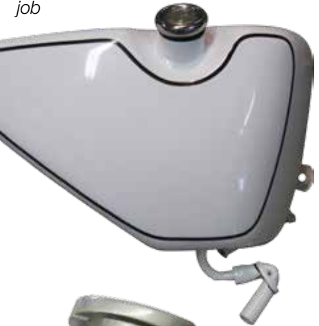
Painting the oil tank was tricky. Any residue oil will screw up a nice paint job
