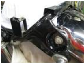
Cut off seat supports seen ahead of fender mount.
