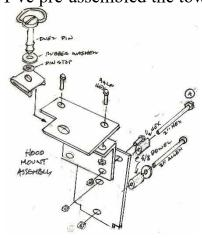
Insert the 2" hex bolt (A) thru the top center hole in your pan and bulkhead. Bolt goes in from the front. Slip on a 5/8 dowel-this goes between bulkhead and assembly. Loose fit the lock nut. Insert Allen screw the same way into the lower center hole.
