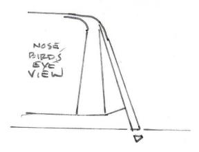
File off the edges of the bumper on the nose. You want the fiberglass angle to match the real aluminum bumper. Align the nose with these mating edges. I supplied six black 1" Allen screws and Nyloc nuts. Mount the nose with them. I've had to use longer ½ screws to pull the nose close on a temporary
