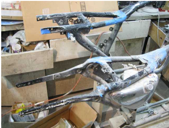
1994-2003 frame in front. 1986 to 1993 frame in rear
